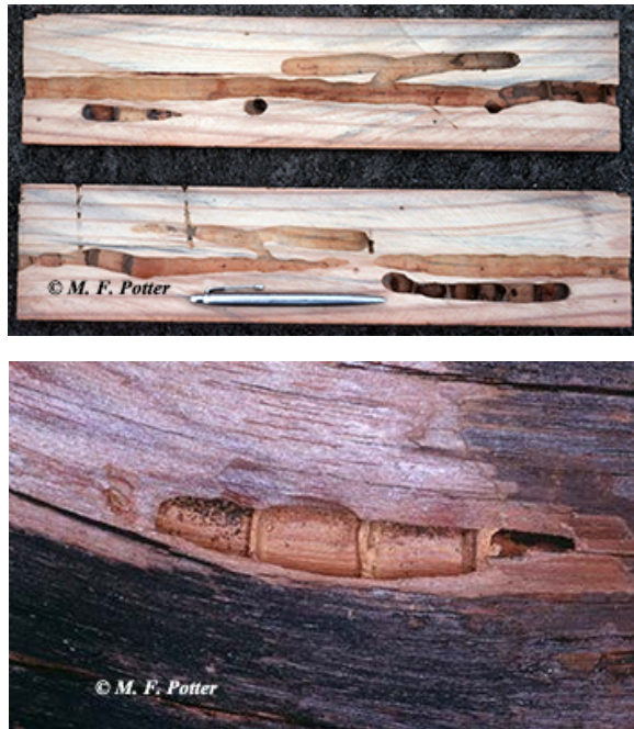
Fig. 3: Cross-section of wood showing carpenter bee tunnels and brood chambers.
