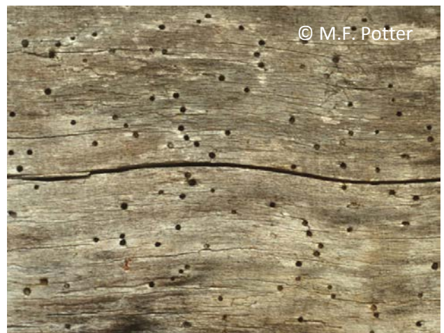
Fig. 6a-b: Active versus inactive infestations. The former usually have fresh powder accompanying the emergence holes.
